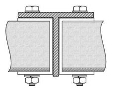
SHOWN: 3-1/4" x 2-3/4" x 1/4" extruded aluminum T-Bar. Bolts 1/4" dia 3-1/2" minimum length. T-bar is available from Acoustiblok Inc. May be bolted, heli-arc welded, or sunk into concrete. 6063-T5 alloy, mill finish, 25 ft, 43 lbs/ea
