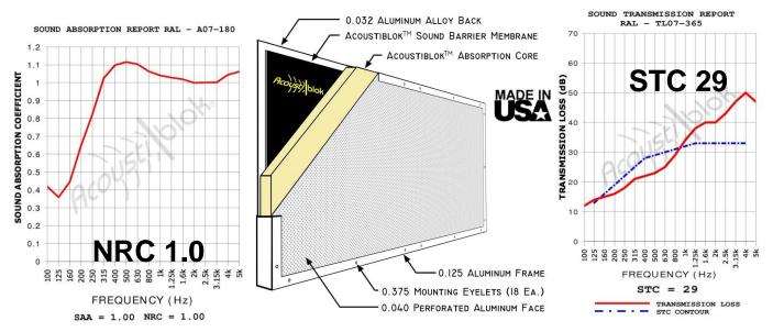
Acoustiblok All Weather Sound Panels<sup>™</sup> achieve high STC and NRC ratings. They have been specifically designed to withstand outdoor exposure in full sunlight, extreme weather conditions, (over 270 mph, 436 km/h wind-tested) and harsh industrial environments. (NRC of 1.0 is the highest sound absorption rating possible)
