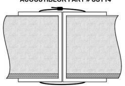
SHOWN: Panels secured side by side with high tensile steel wire ties. Panels may be secured to each other, to fence posts, etc. Calculate the load the wire ties can support from manufacturer's specifications.
