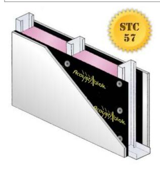
SOUND TRANSMISSION CLASS is a single number that represents the sound blocking capacity of a partition such as a wall or ceiling.
